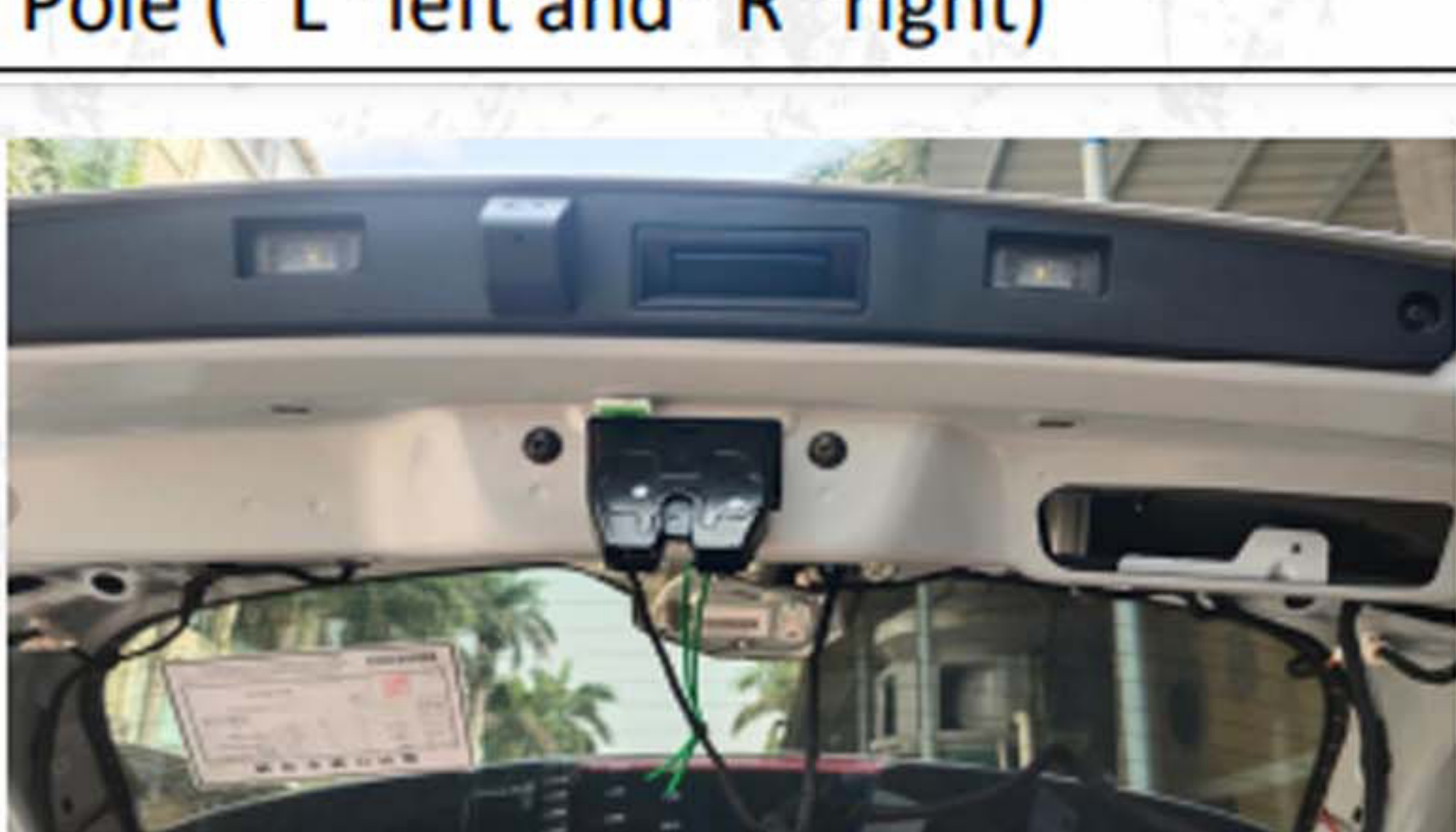
7. Install our equipped locks
