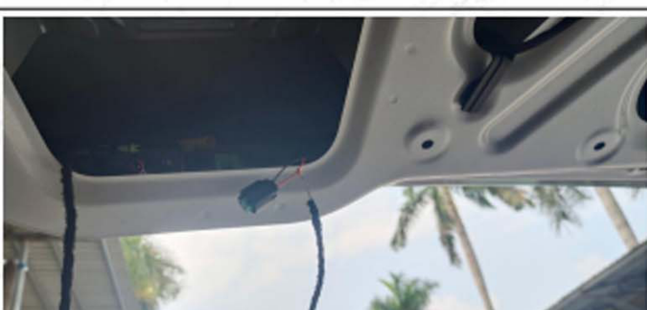
9. The key plug of the original rear door is equipped with us Connect (equipped with harness white wire connect red wire)
