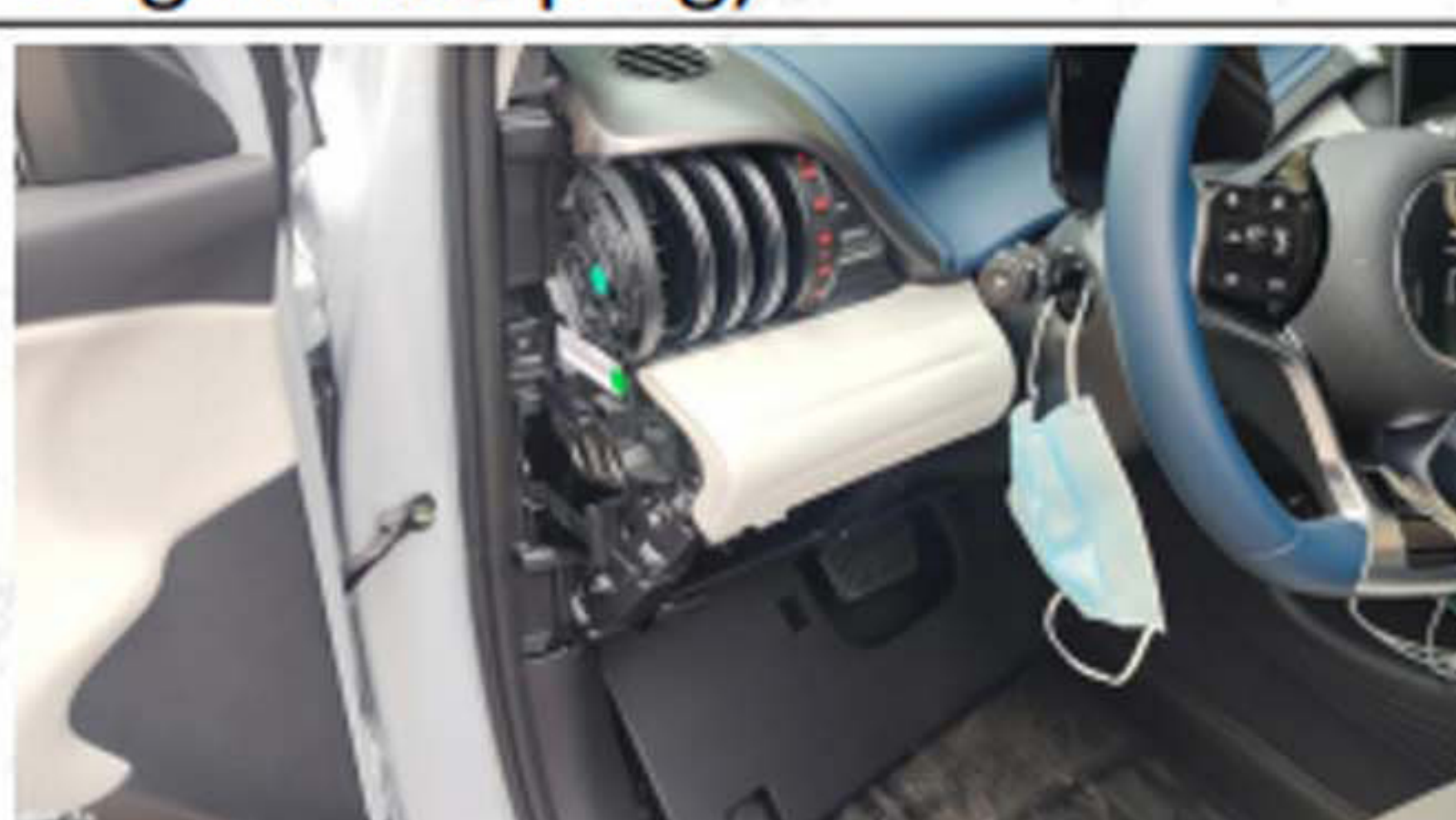
10. Remove the main driver side trim panel
