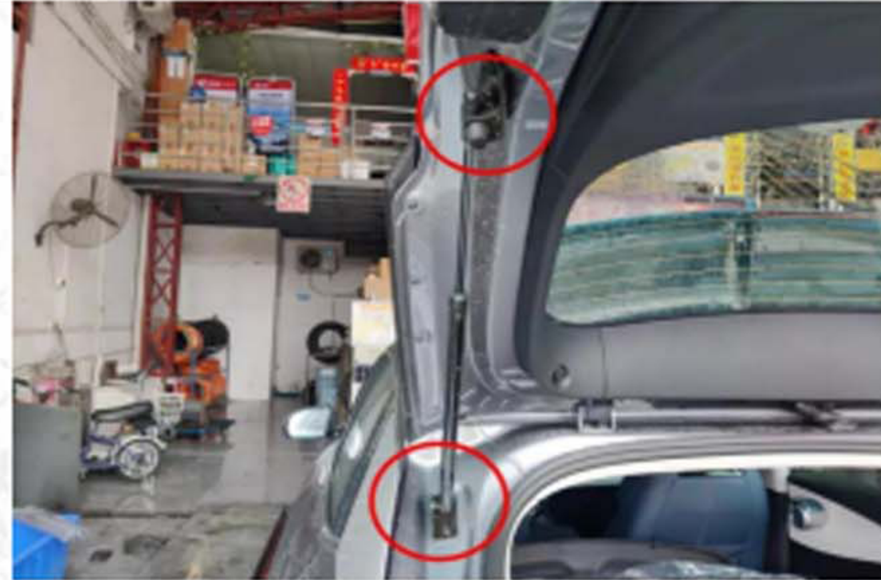
4. Remove the original car pole (left and right sides are the same)
