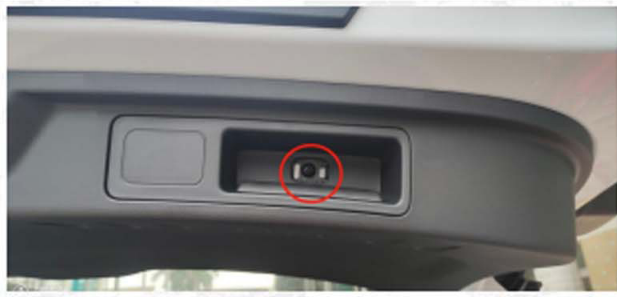
3. Remove the screws of the hand pull box marked in the figure below and remove the hand pull box
