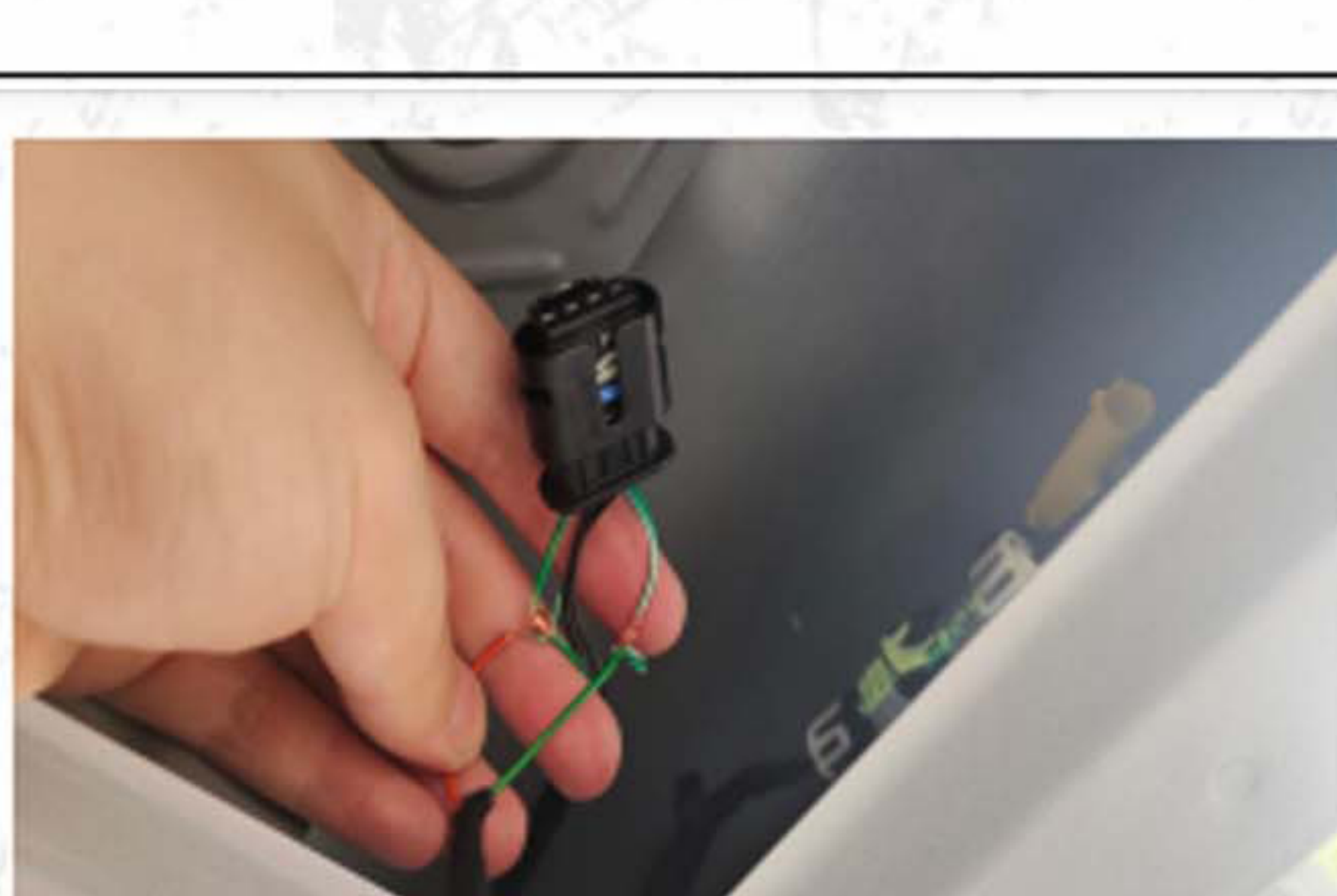
8. Unplug the original car and connect with our wiring harness (match Standby orange wire to connect with the original car plug green wire, green The color line is connected with the green and white side line of the original car plug)
