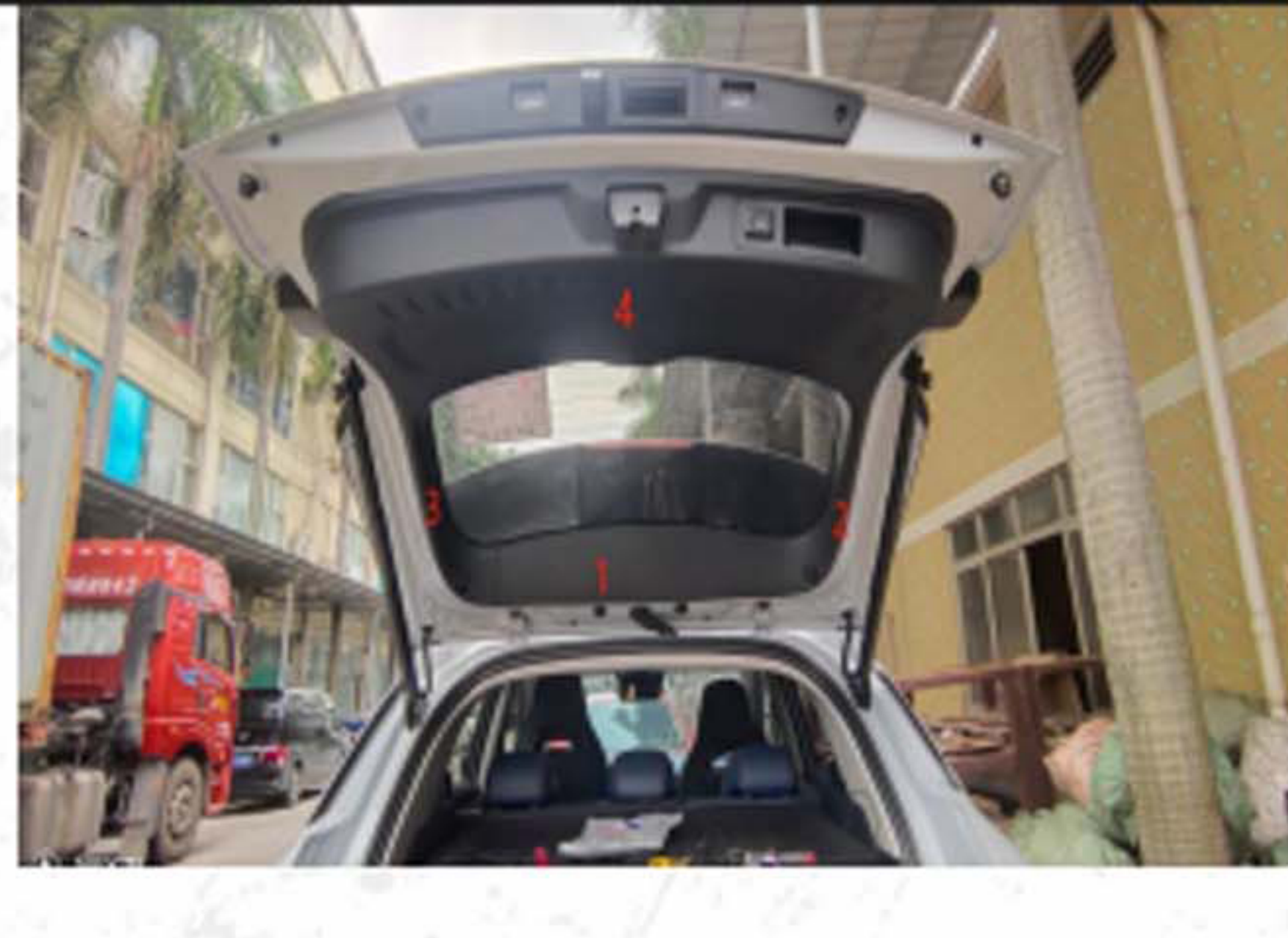
2. Remove the tail door panels according to the figure
