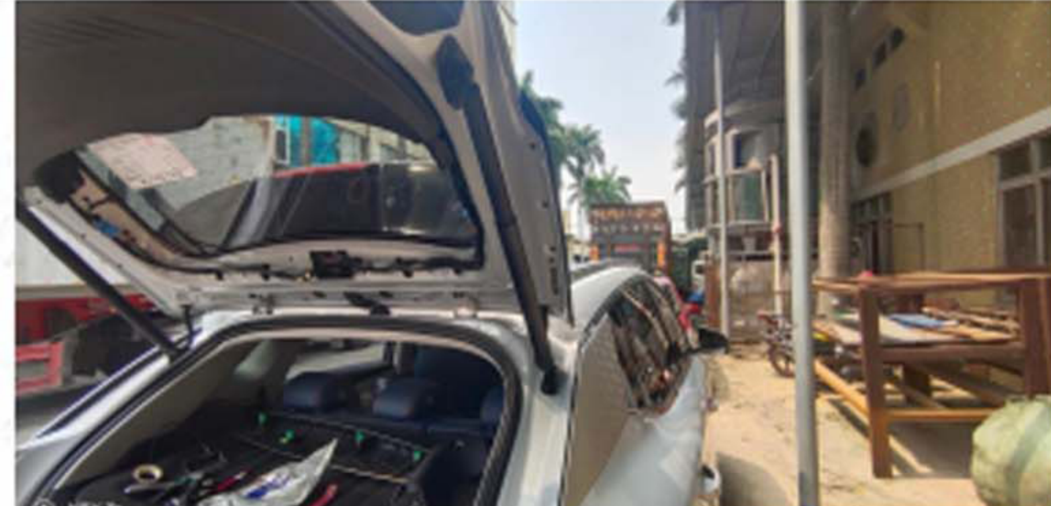
5. Use the original car bracket to install our electric equipment Pole (" L "left and" R "right)
