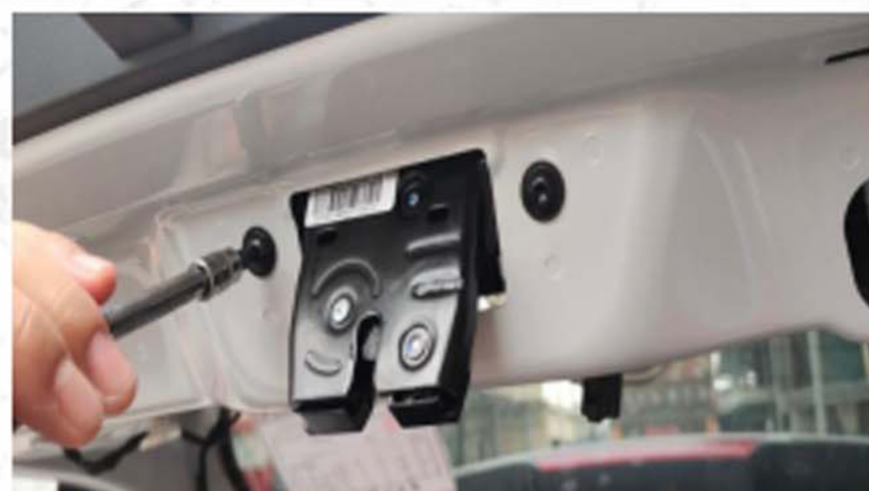
6. Remove the original lock
